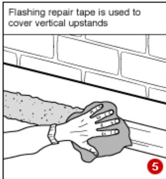
Flashing and joins to vertical upstands can be covered by flashing repair tape. Be sure to apply enough pressure when pressing it in place in order to get rid of any trapped air underneath (5).
